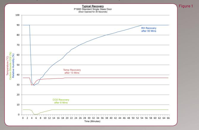
Typical recovery graphs for a LEEC Precision P50 model 3 inner door option fitted:
