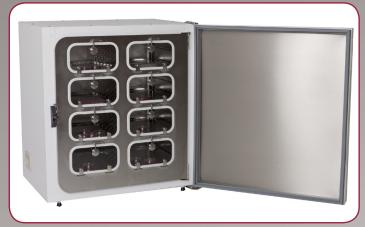
Precision P190D CO<sub>2</sub> incubator with 8 inner glass door option fitted.
